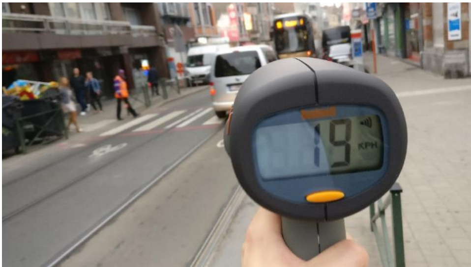
Figure 2 The mobile speed radar used for data collection
