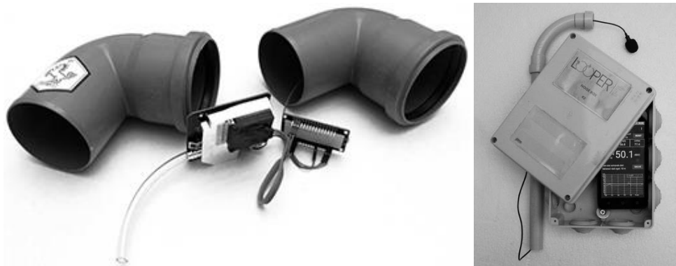
Figure 20 Components from a Luftdaten sensor (left), and a noise box with its waterproof case (right).
